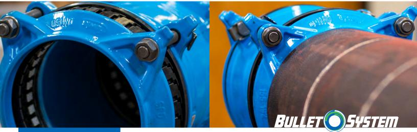
The BulletSleeve by Hawle is an all-in-one socket coupling used to join and restrain steel, DIP, PE/PVC, and AC pipes with corrosion protected connections. Adaptable to varying outside dimensions, ranging from 2- to 16-inches, with a bolt head locking device for one hand tightening. The reusable couplings are rated up to 250psi and carry a 10-year factory warranty. **Reduces installation time** and cost compared to a standard coupling.
